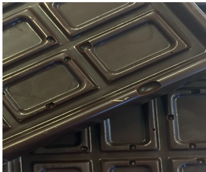
Figure 2: Incorrect viscosity may result in holes in the chocolate.
