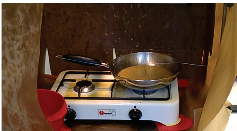
Figure 2: A 'Category 5' margarine with fat-spitting quantities so aggressive that our technologists needed special protection to test them.
