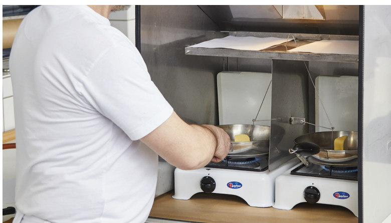
Figure 1: Palsgaard's test set-up for evaluating the spatter of frying margarines. The 'spatter collector' is placed 30 cm above the frying pan. 60 grammes of margarine is heated at max. temperature until all the water has evaporated. Subsequently, the spatter marks on the collector are marked and counted. Tests are performed on various heat sources and with different types of frying pans.
