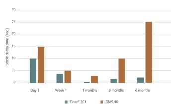
Einar® 201 is an excellent general purpose anti-stat for PP injection moulding applications
